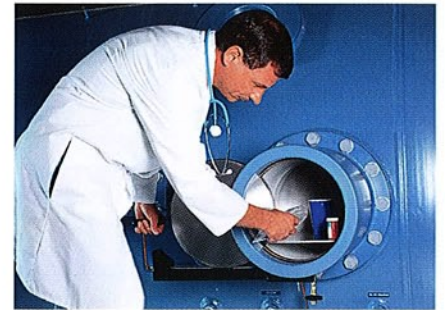
The medical lock is a convenient way to pass refreshments or medical supplies in and out of the system.
